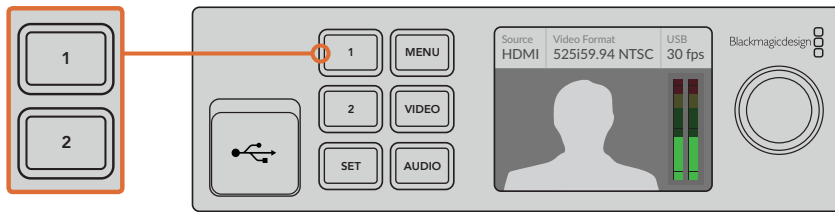
When switching a live broadcast using Blackmagic Web Presenter with a Teranex Mini Smart Panel attached, press the 1 and 2 buttons to switch between the SDI and HDMI inputs
